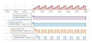
Figure 7: Measurements of consumed power during a test in which the power-to-heat systems have to follow a staircase power profile.
