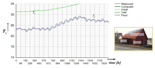
Figure 2. Summer thermal model of RISE experimental villa: The comparison of measurements and solutions of the calibrated model.
