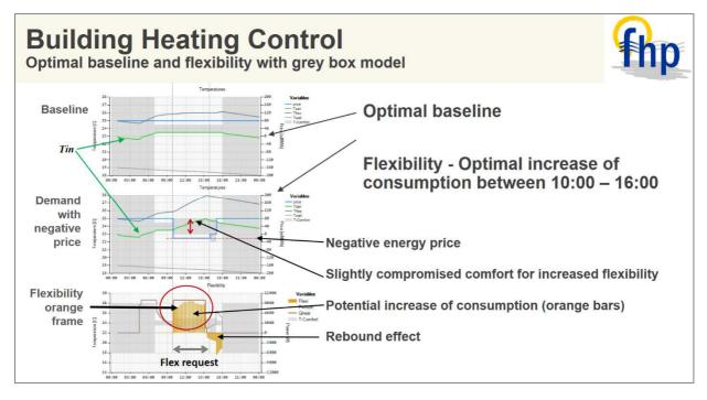
Figure 3. Detected flexibility of building power consumption, which exploits building thermal capacity. Flexibility enablers are varied energy price and relaxed thermal comfort
