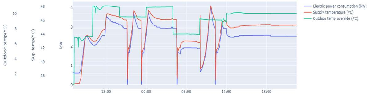
**Figure 16: The response of the electric power consumption and supply temperature to the control signal.**
