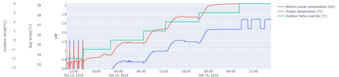
**Figure 14: A zoomed in version of the ramp up test, to focus on the delays in response of the supply temperature to change in outdoor temperature.**
