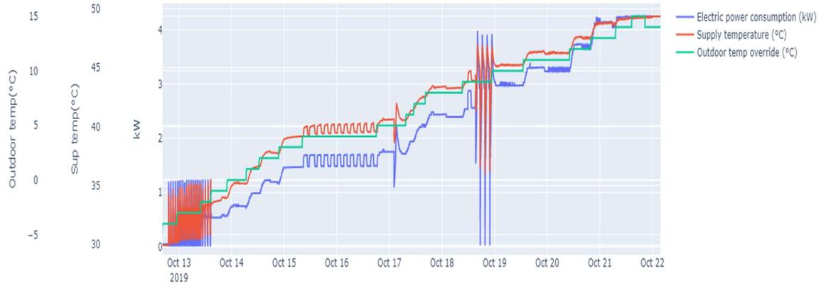
**Figure 4: Ramping up test: the response of the electric power consumption and supply temperature to changes in the outdoor temperature override.**
