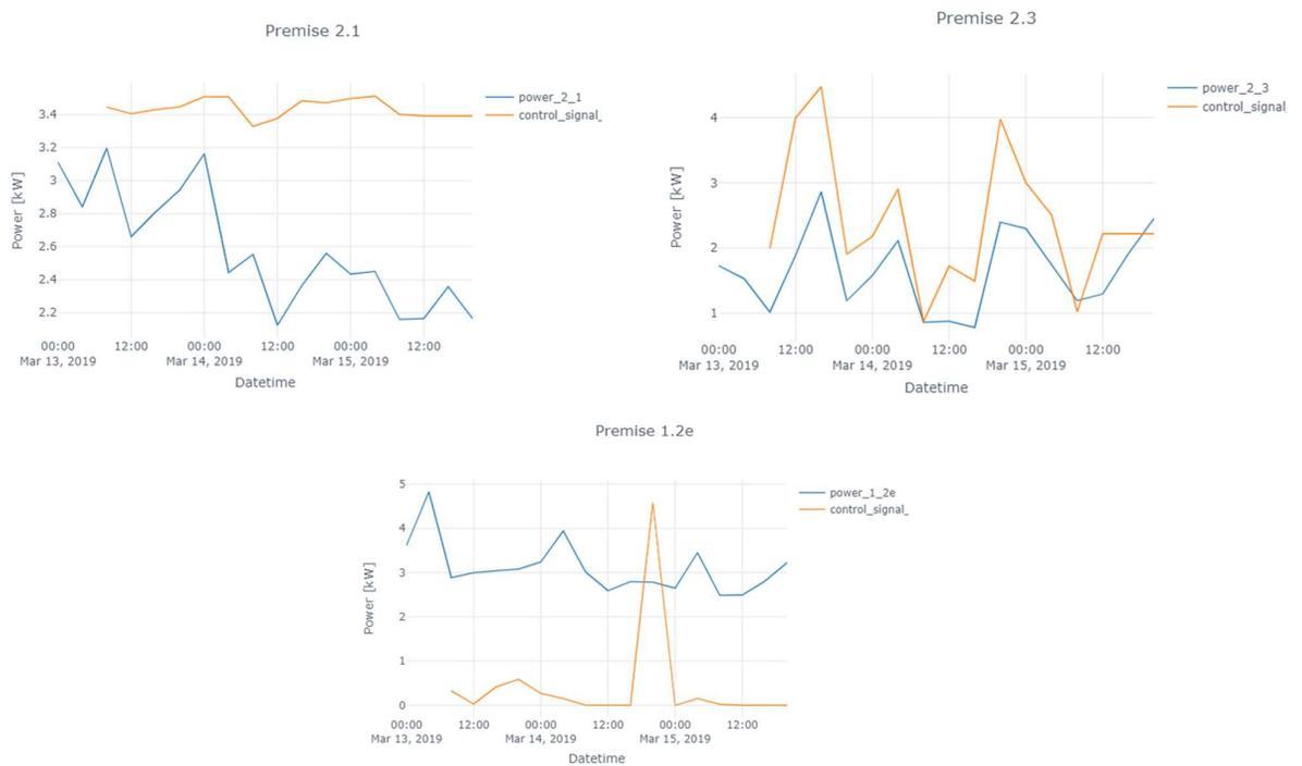
**Figure 29: Comparison building control signal<sup>8</sup> and actual power consumption of the buildings in test Flex\_1 (4-hour average).**
