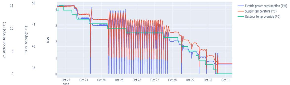
**Figure 6: Ramping down test: the response of the electric power consumption and supply temperature to changes in the outdoor temperature override.**
