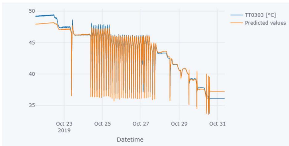
**Figure 12: Validation of the model in ramping down test.**
