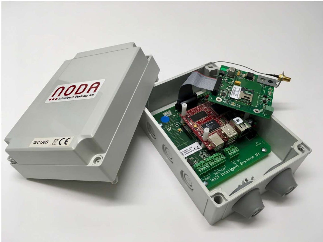
Figure 25 The NODA Integrated Energy Controller.
