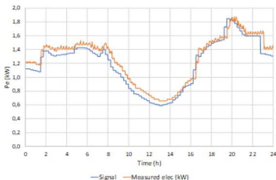
Figure 3: 24h-profile based on profiles used in Karlshamn (with some adjustments) tested in lab using direct control.
