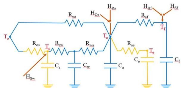
Figure 1. RC schema of the gray-box model with five temperatures as state variables  $T$ . Basic blue model is extended by two additional states in yellow.
