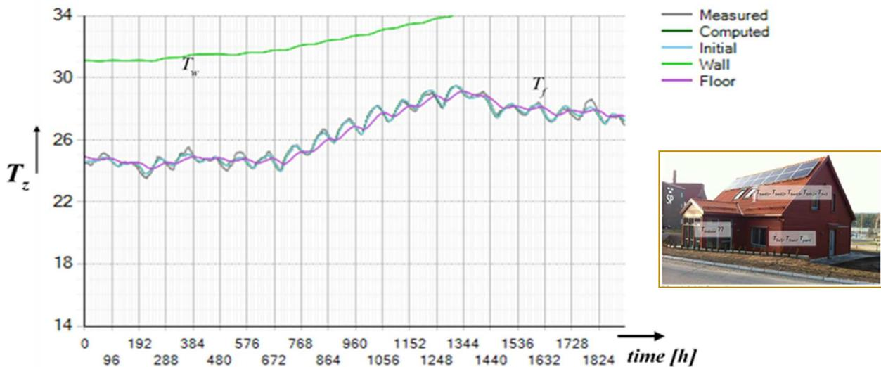
Figure 2. Summer thermal model of RISE experimental villa: The comparison of measurements and solutions of the calibrated model.
