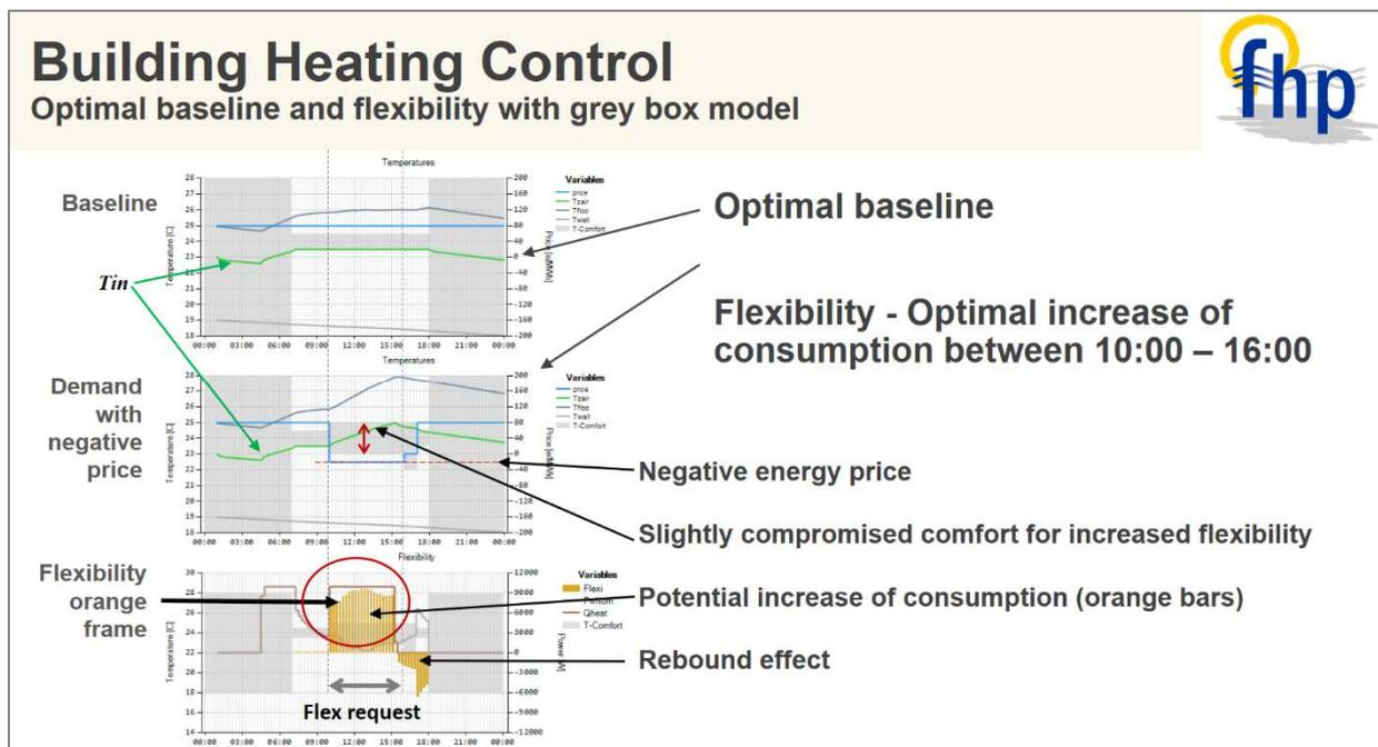
Figure 3. Detected flexibility of building power consumption, which exploits building thermal capacity. Flexibility enablers are varied energy price and relaxed thermal comfort
