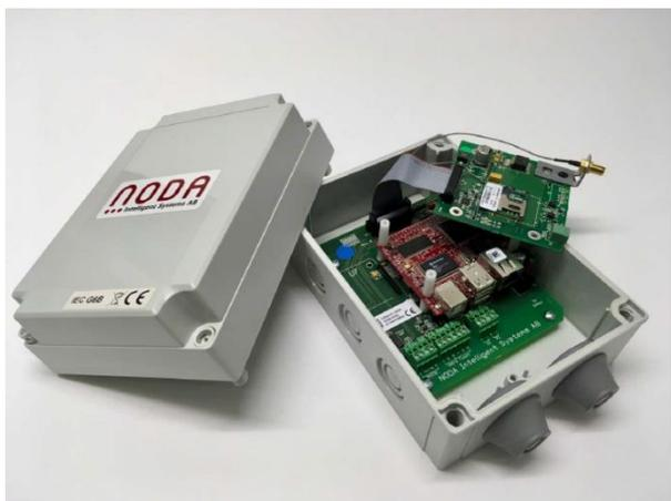
Figure 2: The sensor-override hardware used for the installation in Karlshamn
