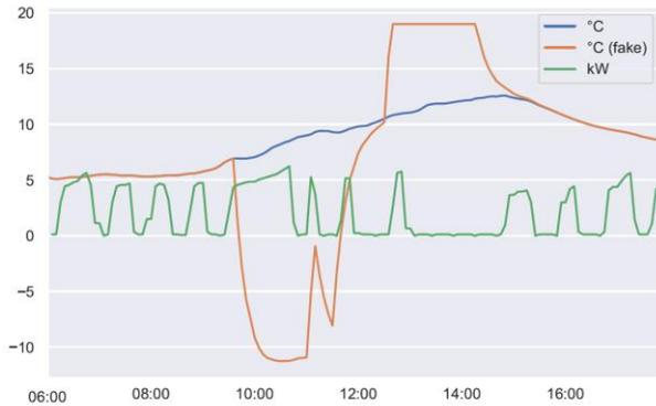
Figure 3: Example of control actions in a building with a heat pump. The blue line is the actual outdoor temperature and the brown line is the overridden outdoor temperature that the controller reacts on. The green line is the power demand of the heat pump.
