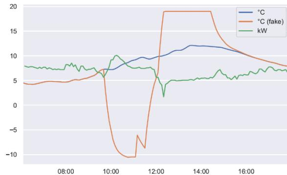
Figure 4: Example of control actions in a building with a heat pump. The blue line is the actual outdoor temperature and the brown line is the overridden outdoor temperature that the controller reacts on. The green line is the power demand of the heat pump.
